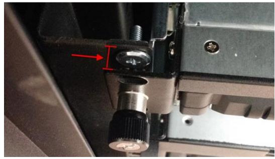
If the spacing is bigger than 1/8", chassis cannot be secured to cabinet due to too much spacing between L bracket and rackmount flange.
