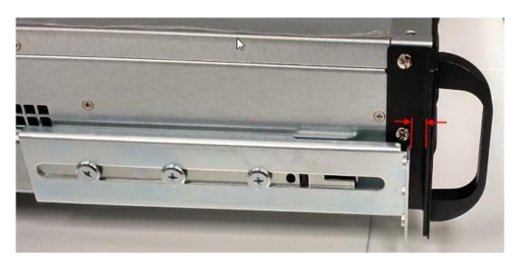
If mounting posts distance is 29" or under, ensure the spacing between L bracket and rackmount flange is no bigger than 1/8" (can be zero), otherwise chassis cannot be secured to cabinet's mounting posts. See below image
