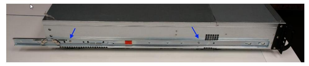
1. Install and secure inner rails to chassis with two screws on each side
