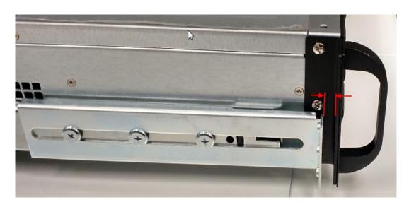
If cabinet mounting posts distance is 29" or under, ensure the spacing between front L bracket and rackmount flange is **no bigger than 1/8"** (can be zero), otherwise chassis cannot be secured to cabinet's mounting posts. See below image
