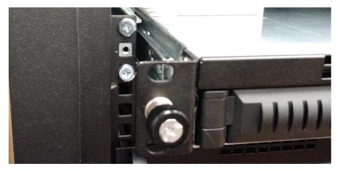
4. Secure chassis to cabinet via thumb screws when needed
