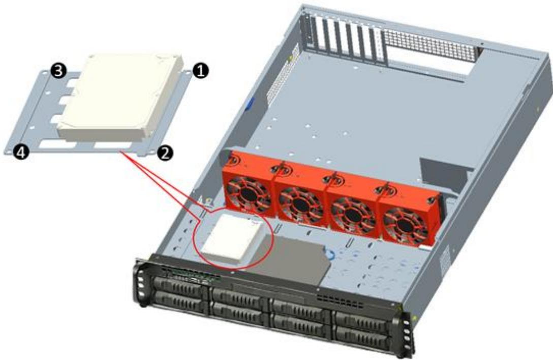
3. Install HDD bracket onto chassis
