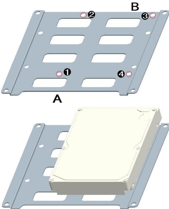
2. Install 2.5" HDD/SSD onto HDD bracket
