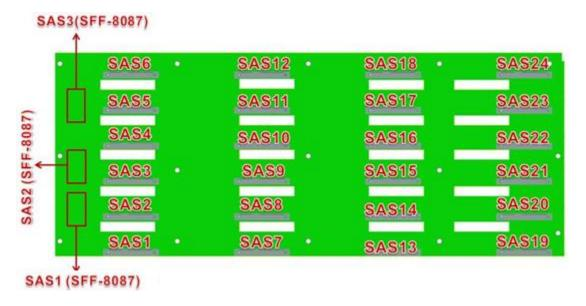
1. Only need to connect one of the three connectors from the front 24-bay SAS expander backplane to a controller to access all 24 hard drives. Try with different connectors if the controller doesn't not recognize the SAS expander backplane.
