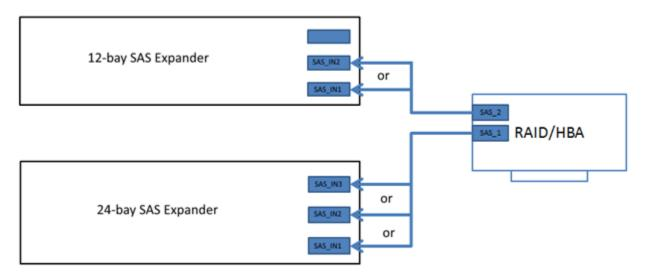
Connection Diagram of Controller and SAS Expanders
