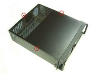
2. Remove the screws to remove the drive bay cage.
