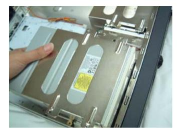
7. Install motherboard and plug in all the USB cable and Front Control connector. The USB connection is on the accessory box.
