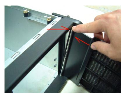
9. Make sure the door is secured and locked up in the holes.
