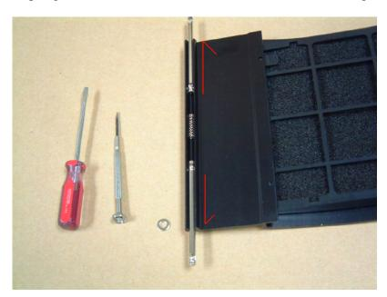
5. Put the spring and the hinge to the door that you want to install.
