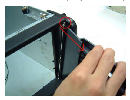
4. Take the hinges and the spring out from the trench. Please notice that there is a ring on bottom of the hinge.
