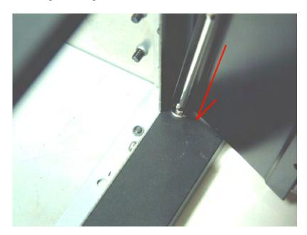
8. Push the top of the hinge and push it into the lockup position. You should hear an click sound if the hinge falls into the right position.
