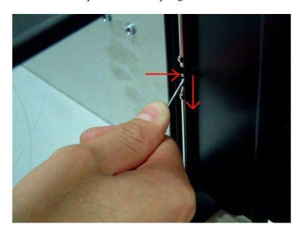
2. Hold the spring down and use another screw drive to push down the hinge.
