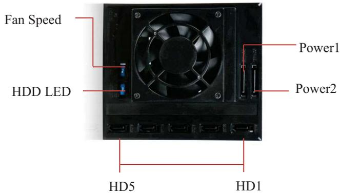
**HD1—HD5:** SATA 7Pin data single connector for SATA or SAS primary channel connections
