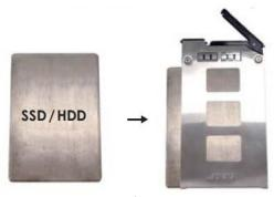
Insert slim 2.5" SSD/HDD into the tray.
