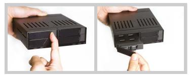
2) Place HDD/SSD onto the tray, and use M3 countersink screws to secure the HDD/SSD.
