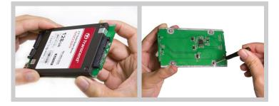
4) Insert the PCB back to the HDD enclosure and secure the back cover with screws.
