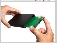
3)Place HDD/SSD onto the PCB, and connect to SATA connector. Use M3 screws to secure the HDD/SSD.
