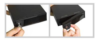
2) Slide a 3.5" HDD into the BPX-525-SA, then close the door and lock it.
