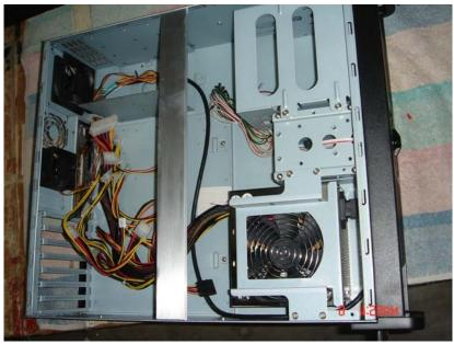
Mount the whole power supply with bracket back to the chassis.
