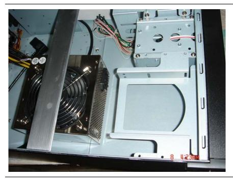
Remove the top panel and place the power supply.
