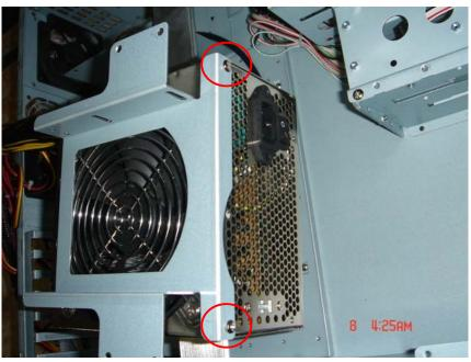
Remove the bracket and mount the bracket on the power supply.
