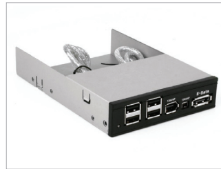
RP-HUB-SAUF 3.5" Combo Hub for USB2.0/ Firewire/ e-SATA
