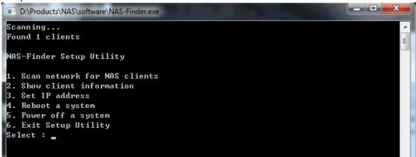
NOTE: eth0 must be connected in order for the NAS-Finder to scan and find an IP address.
