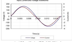
Input AC Current Waveform (ITHD = 6.45%, 50% Load)
