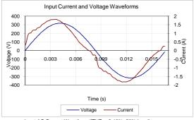
Input AC Current Waveform (ITHD = 8.46%, 50% Load)
