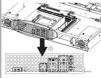
2. Loose 2 screws to remove IO shield
