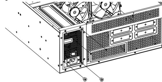
1. Loose 4 screws on the PSU bracket
