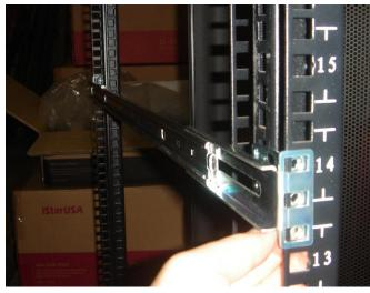
c. Fasten the brackets onto the rack. (Use M5 Screw)
