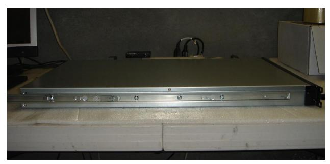
3. Mount the L shaped bracket onto the outer channel. (use black round head screw)
