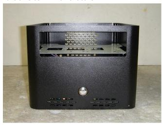
2. Mount brackets (DD-BRT-S0512) on the two sides of the 5.25" HDD Cage
