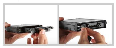
2) Slide HDD into the tray, and make sure the HDD is secured with plastic latch installed.
