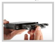
3) Hold down plastic latch and release HDD from the rear (Image 3.1) or unscrew HDD (Image 3.2)
