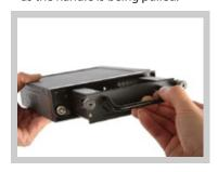
3) Hold down plastic latch to release HDD from the rear.
