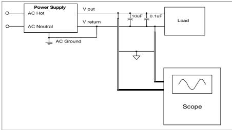
Figure 1. Ripple voltage test circuit
