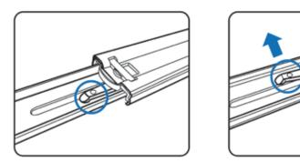
You will see a locking clip at the end point of the center slide. Push it down and unlock the center slide.
