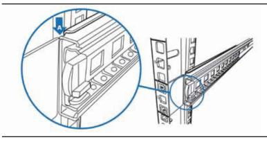
Align front outter rail to the indent of L bracket between Point A & B.
