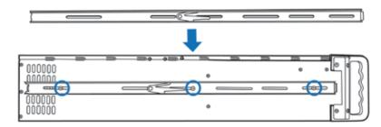
Now put the center slide right next to the rackmount chassis. You should be able to find screw holdes on both sides of the chassis. Holes are used for mounting the center slide. Later, the center slide will be use for attaching the sliding rail.
