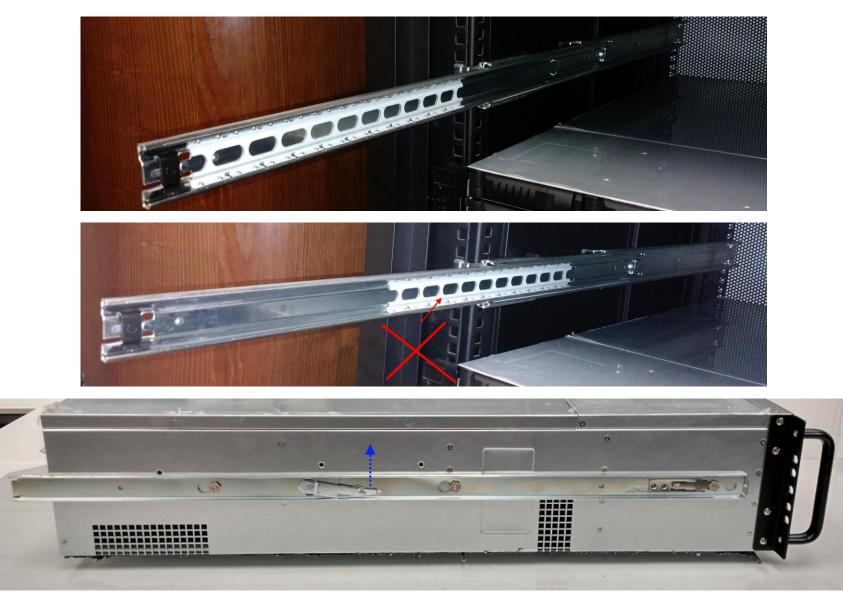
4. Pull the rails (middle rails) all the way out from cabinet and pull one side latch **up** and push the other side latch **down** at the same time when sliding chassis in or releasing chassis from rails.
