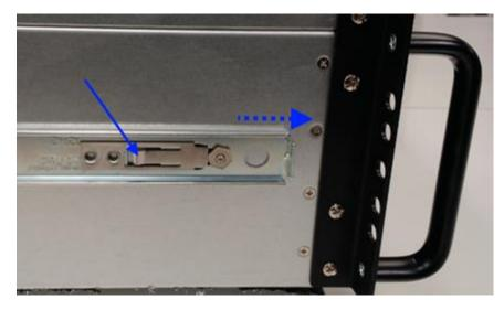
To release inner rails, push the latch and push the inner rail forward
