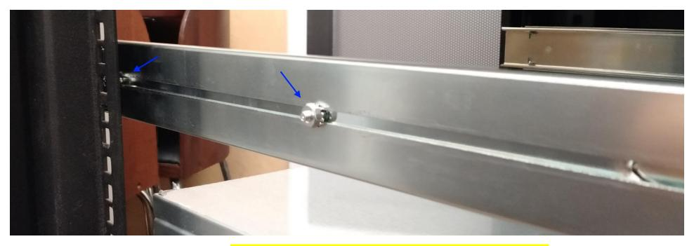
3. After rails are mounted onto a cabinet/rack, make sure use tools to tighten the nuts that are loosened in previous step.
