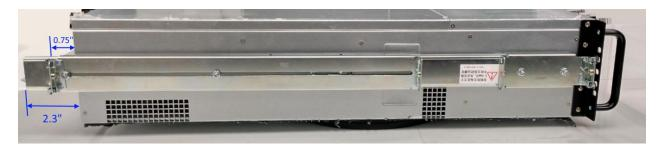
Outer rails stick out 2.3" from rear end of chassis when rails are mounted with minimum mounting distance 26.5"
