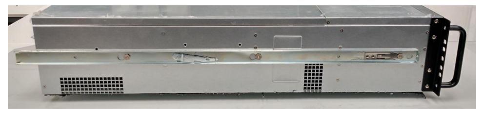
1. Install and secure inner rails to chassis.
