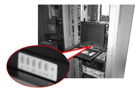
2.10 To return the drawer back to the unit, fold screen down and push in the 2 tap located on each side of the rail then push the drawer back in.
