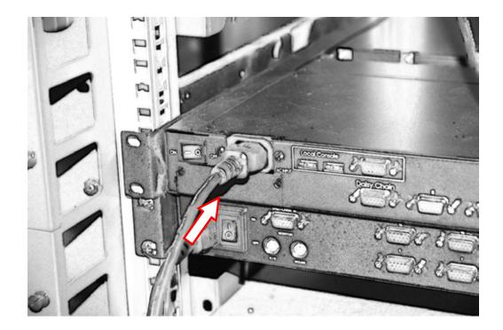
2.5 Connect the host cable to the rear of the drawer. For the WL-21701, USB type can be connected to its single port. For WL-21708/21716 both PS/2 and USB type can be use with the KVM, just choose the desire type to match with your system, the KVM accepts both. Refer to Section 3 for further detail. (\*WL-21708 Shown)
