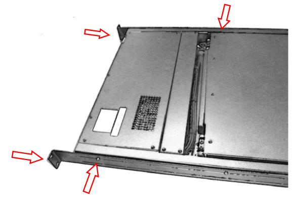
2.3 Secure the rear and front rack mounting to properly mount and fix its position into the cabinet.
