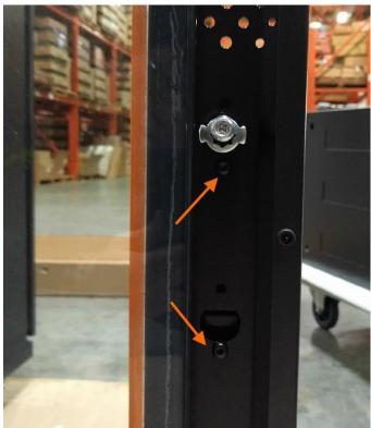
9. Install tongue. Make sure it is in correct open and close position
