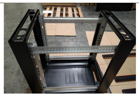
6. Put on top cover and secure it with the same (8) screws and (8) nuts as the base does.
