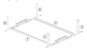
3. Using the remaining two Beams assembled in step 1, line up the other set of Left and Right Vertical Rails and fasten them to the Base and Top Brackets as shown.
