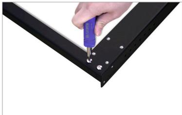
Joint long horizontal bars (A) and short horizontal bars (C) together.
