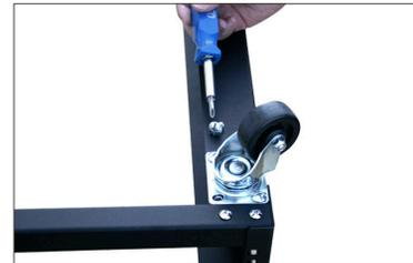
Install the 4x castor (E) with 16x screws. (F)
